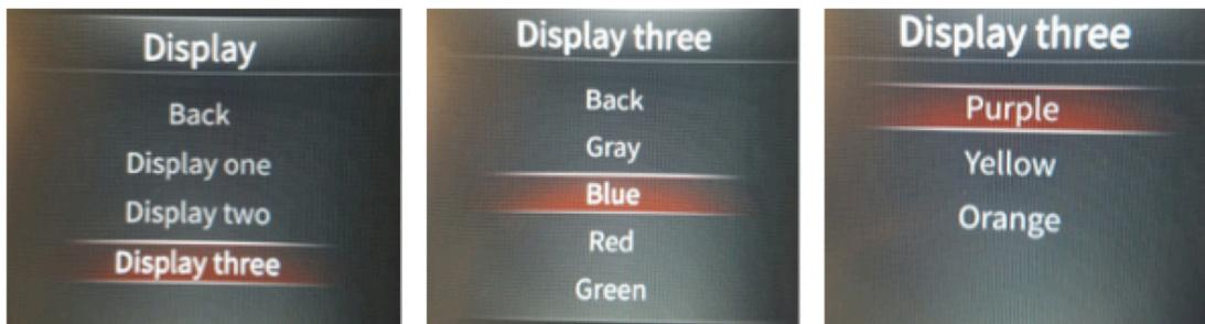
**To Exit**, simply scroll up to Back, and press Enter., then scroll up to Back on the Display menu, and press Enter, then scroll up to Close on the Main menu and press Enter.
