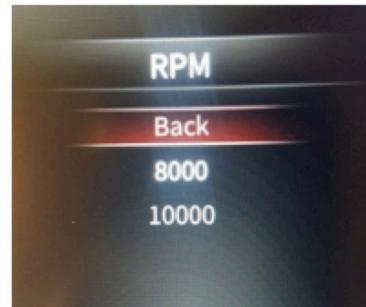
Once you have chosen the Tachometer Scaling, simply scroll up to Back, and press Enter. Then, scroll to the top until Back and press Enter. Next, once you are back into the Main Menu, scroll up to Close and press Enter.
