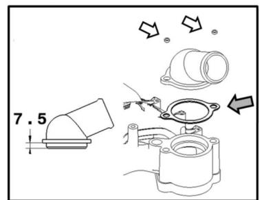
4. Use (2) coolant cap bolt spacers (White arrows) if the removed manifold coolant crossover is made of plastic. These parts are not necessary for aluminum crossover.
