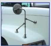
Reinforcement of high-stress areas where objects will be mounted, such as mirrors and door handles
