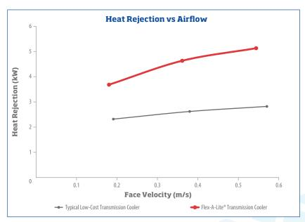
The heat rejection of the new Flex-A-Lite® transmission cooler is nearly double that of the a typical low-cost transmission cooler.
