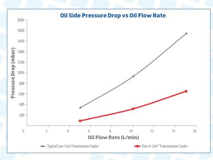
The oil pressure drop of the low-cost transmission cooler is near 2.5 times greater compared to the Flex-A-Lite® transmission cooler.
