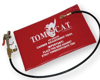
Makes camber adjustment a one-man job. Works on many GM and Chrysler vehicles using two-bolt lower strut mounts. Inflatable air bladder fits between tire and strut for easy and controlled adjustment of camber settings.
