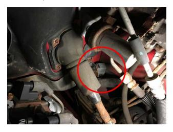
16. Locate the 24-pin connector for the air suspension module. It is located at the rear of the vehicle, near the trailer hitch, and behind the rear differential housing. Remove the red plastic retaining clip and then the 24-pin connector. Place the remaining bag and zip tie over the connector to protect from contaminates.
