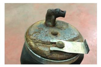
4. Disconnect the air lines from the height control valve near the left rear frame rail and spare tire. Squeeze the tabs on the air line connector and pull out of the way. Then insert Toyota tool SST 09730-00010 to expand the claw in the housing and pull out the air line (or cut the air line). This will deflate the air springs.
