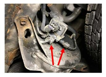
5. Remove the air spring assembly along with the air line.
