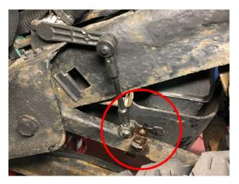
6. Remove the bolt that holds the brake line bracket to the rear differential.
