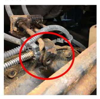
7. Disconnect one end of both rear anti-sway bar end links.
