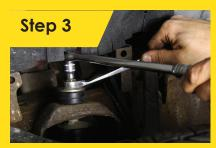
Finally, use a ratchet to hold the bit in place and a wrench to tighten the nut.
