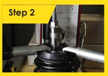
Next, find the corresponding passthrough socket and slide it over the top of the bit and onto the nut.
