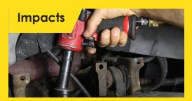
Shock absorbers are built with an internal piston nut designed to hold valving together inside the unit. Any rapid spinning of the rod – like that which occurs when using an impact to install or remove the external mounting nut – can cause it to come loose. This can dislodge the rod and damage internal components.
