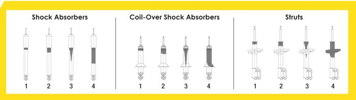
Oil found on units 1 and 2 reflect weepage and do not require replacement. Units 3 and 4 reflect leakage and require replacement.
