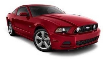
This refinish repair consists of a tri-coat process made up of a red metallic ground coat layer, a tinted translucent mid-coat layer followed by a final clearcoat layer. See illustration below.
