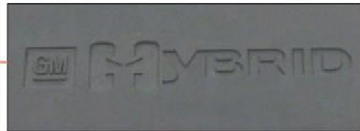
A Hybrid Logo Is Imprinted On The Battery Case Which Indicates That Intermediate Voltage Is Contained Within.
