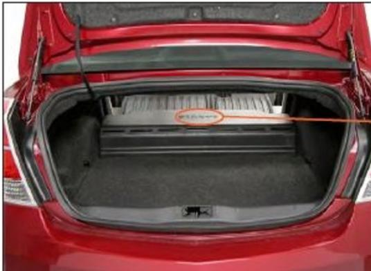
The 36 Volt Nickel Metal Hydride Battery Pack Is Mounted In The Trunk Compartment Behind The Rear Passenger Seat.
