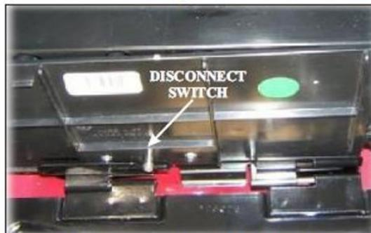
Swing The Cover Down And Slide It To The Left To Remove It. Once The Cover Is Away From The Hybrid Battery Case, The Disconnect Switch Automatically Disconnects From The Rest Of The System. Wait about 15 minutes for the system to fully discharge.
