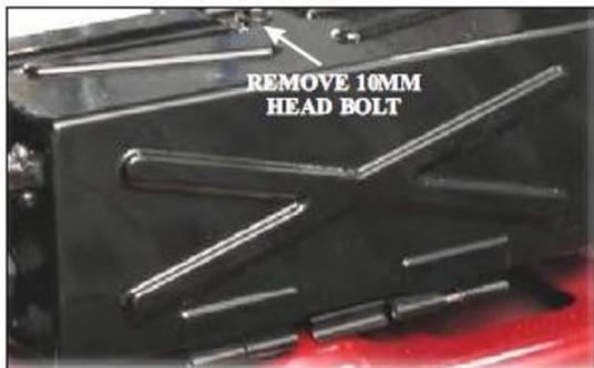
Remove The 10 MM Head Bolt From The Battery Disconnect Switch Cover While Wearing Protective Rubber Gloves.
