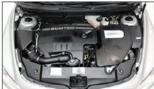
Remove The Generator Control Module Cover In Order To Provide Access To The Module In Order To Permit Voltage Checks.
