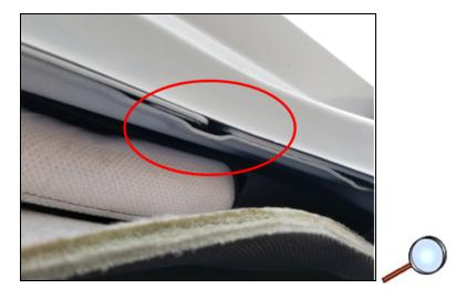
4. Locate the crease/gap in the sheet metal.
