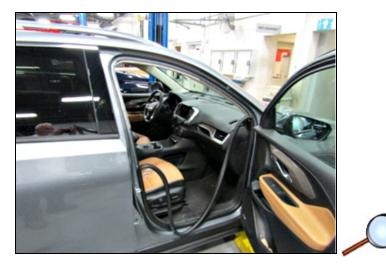
2. Partially remove the front side door weatherstrip (body side) from the front door radius.
