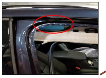
3. Locate the sheet metal area at the rear radius, shown in the graphic above.
