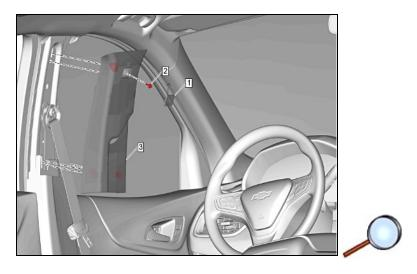
1. Detach and partially remove the center pillar upper trim panel (3) on the affected side(s). Refer to Center Pillar Upper Trim Panel Replacement. in SI.
