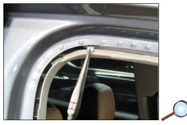
9. Apply SEM 39337 Door Skin & SMC Adhesive, or equivalent, to each side of the metal piece, then using pliers, or other suitable tool, wedge it into the widened sheet metal crease.
